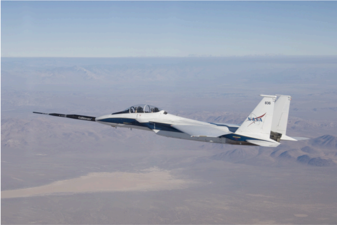
Figure 1. NASA F-15B modified with Gulfstream Aerospace Corporation Quiet Spike™ shown in the fully extended position.
