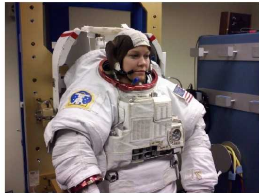
Figure 3. Dr. Moore in the HUT, with the HUT-to-LTA body seal closure locked. Before pressurization can occur, the right glove and helmet will be installed. Photo contributed from Sandra K. Moore personal archive
