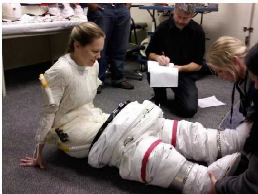
Figure 2. EVA Task instructor Dr. Sandra Moore donning the LTA during the third fit check session. A suit technician assists Dr. Moore by manipulating the LTA's inner bladder, to clear space for Dr. Moore to insert her foot into the boot. Photo contributed from Sandra K. Moore personal archive
