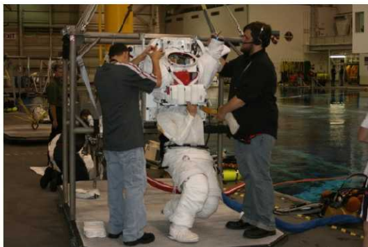
Figure 5. EVA Task instructor Matthew Gast donning the HUT, which is mounted to the lifting platform, prior to a training session in the NBL. Photo contributed from Matthew Gast personal archive
