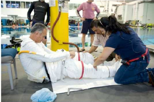
Figure 4. Astronaut John “Danny” Olivas donning the Lower Torso Assembly (LTA) on the NBL pool deck. The “L” shaped handle on the floor to his immediate right is installed on the body seal closure and is used to aid in mating the LTA body seal closure to the Hard Upper Torso (HUT). Source: jsc2009e061367.jpg (photo added 03/25/2009)
