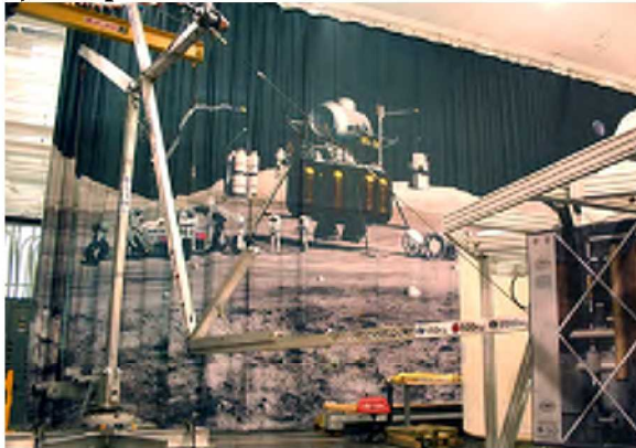
c) Fork-lift mode, reaching under lander mockup. Figure 3. LSMS configurations.
