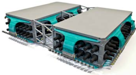
Detector configuration of the Super-TIGER instrument. Credit: NASA/Super-TIGER
