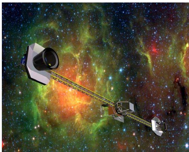
SPIRIT, shown in this artist's concept, is a structurally connected far-IR interferometer for imaging and spectroscopy. Credit: NASA/GSFC
