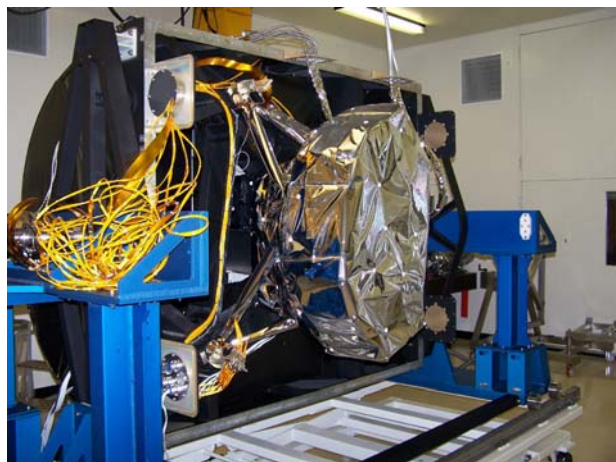
An engineering model of the Mid-Infrared Instrument went through thermal vacuum testing in 2008
