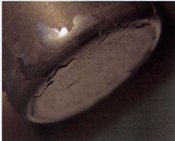
Figure 7. Post-test images of NbC coated high density graphite specimens following hot hydrogen exposure. Note premature spallation due to thermal shock.
