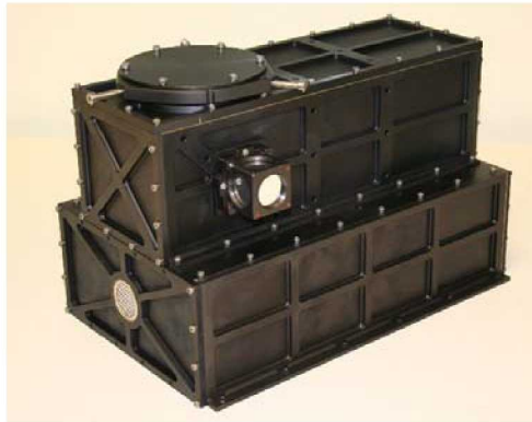
FIGURE 1. Next Generation Advanced Video Guidance Sensor (NGAVGS) Block II Prototype
