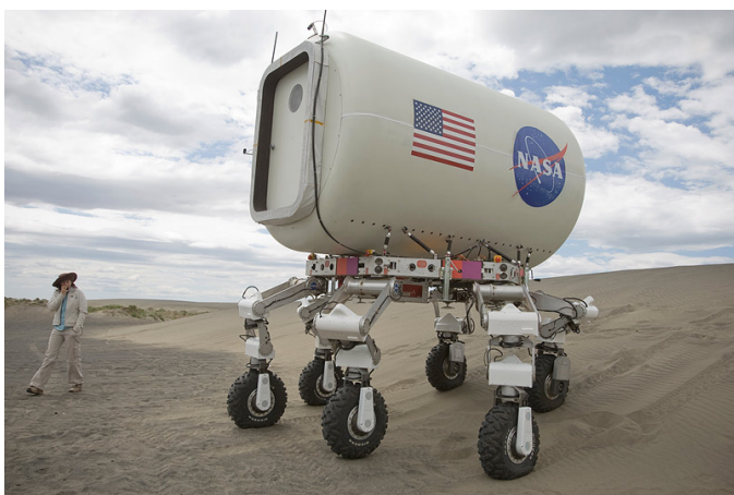
NASA's test version robotic mobility system ATHLETE (All-Terrain Hex-Legged Extra-Terrestrial Explorer) carrying a lunar habitat module during tests of future moon systems at Moses Lake, Washington. Photo from NASA Jet Propulsion Laboratory public web site.
