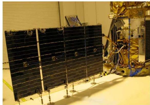
Figure 11 SADA Integrated onto Glory during Solar Array Deployment Testing
