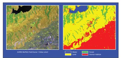
This False-Color Image and Classification Map were derived from image data acquired by an airborne visible/infrared imaging spectrometer (AVIRIS) over Moffett Field, California. The classification map is typical of images meant to be processed by use of the present algorithm.
