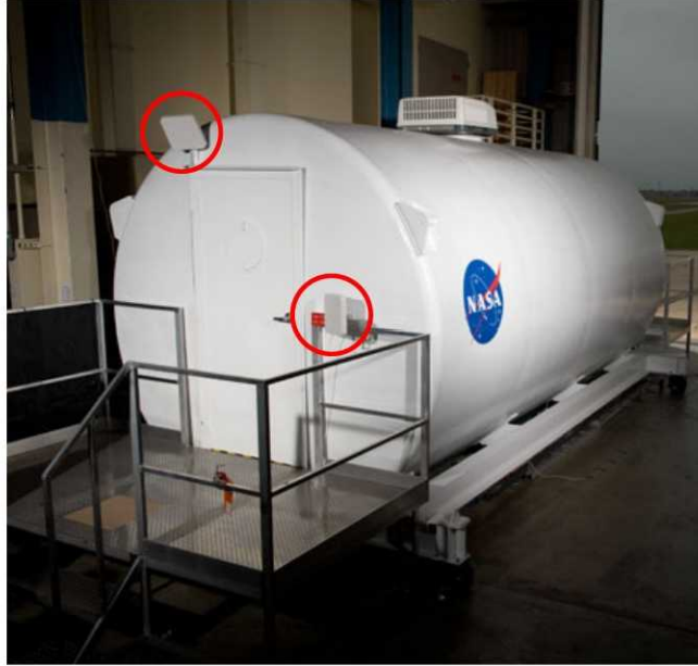
Figure 4. Lunar Habitat Wireless Test Bed (LHWT) with exterior RFID antennas (red circles) at first portal.
