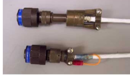
Fig. 5 EMI and standard pigtail connectors
