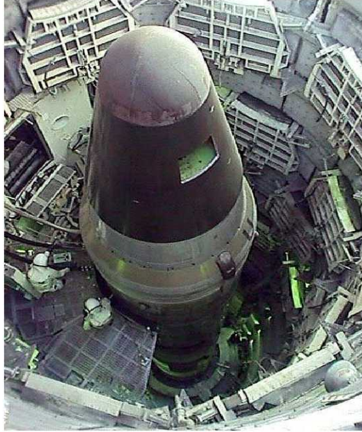
Figure 7-1: Technicians Working on Fold-Down Platform in Titan Silo Level 2
