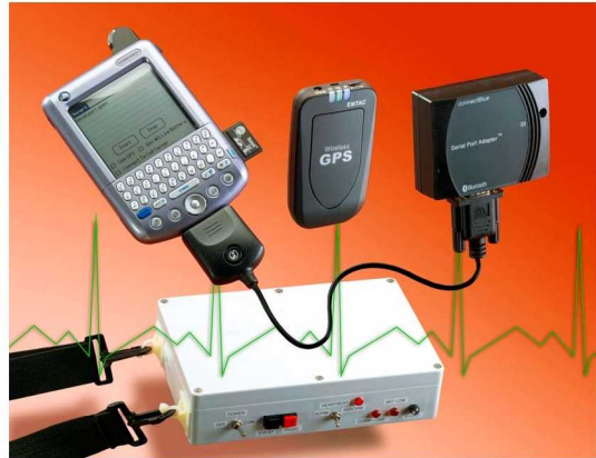
Figure 7.—Researchers will test this prototype of the heart monitoring system for ambulatory patients with arrhythmia symptoms.
