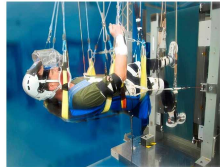
Figure 1.—The enhanced Zero-Gravity Locomotion Simulator (eZLS) at NASA Glenn.
