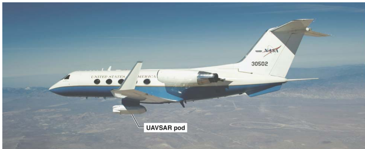
Figure 1. NASA Gulfstream III jet carrying miniaturized polarimetric L-band synthetic aperture radar.
