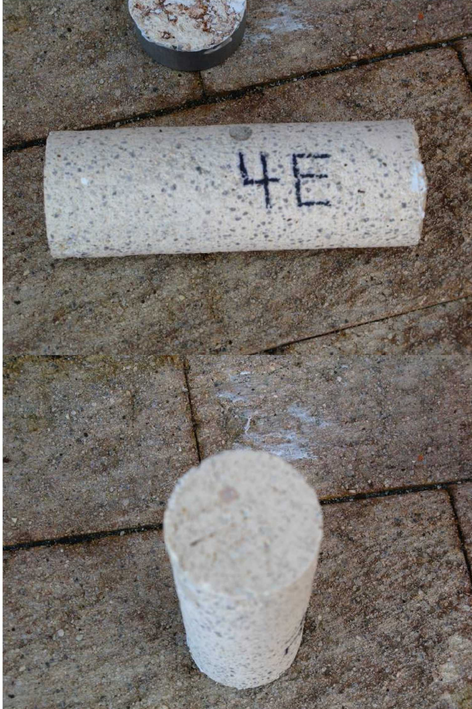
Figure 14. Core 4E – side image of core and back end of core, closest to the concrete wall
