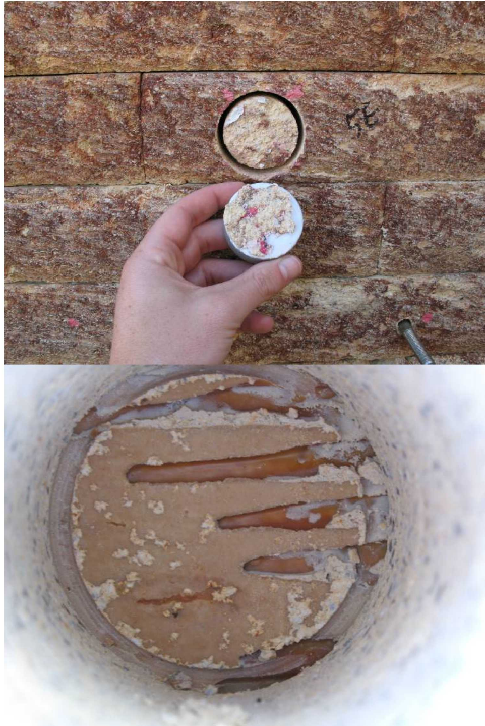
Figure 17. Core 5E – successful test: failed at 82 psi (pull stub and core face and the image inside the brick after the core was removed)
