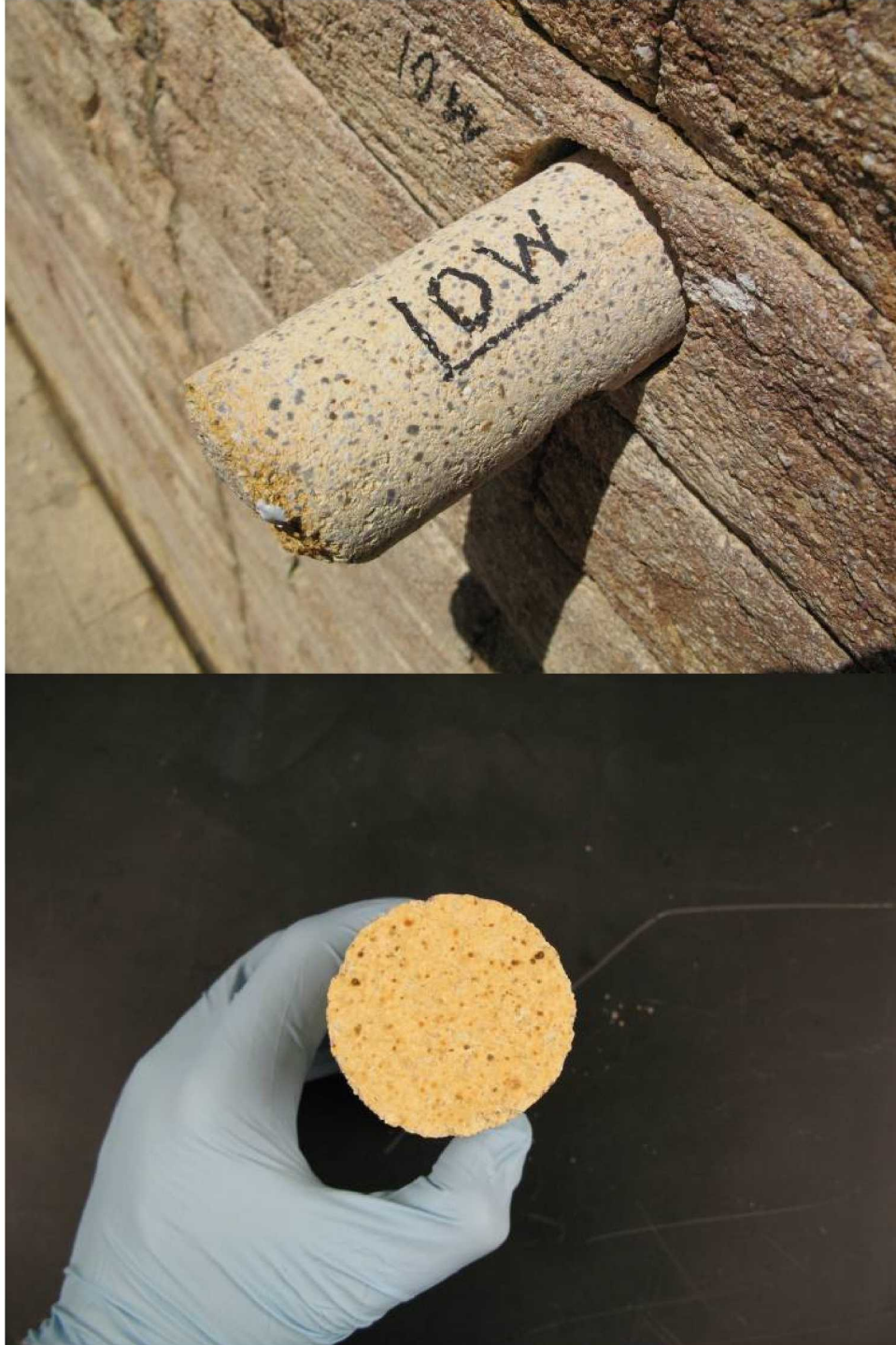
Figure 38. Core 10W – side image of core and back end of core, closest to the concrete wall
