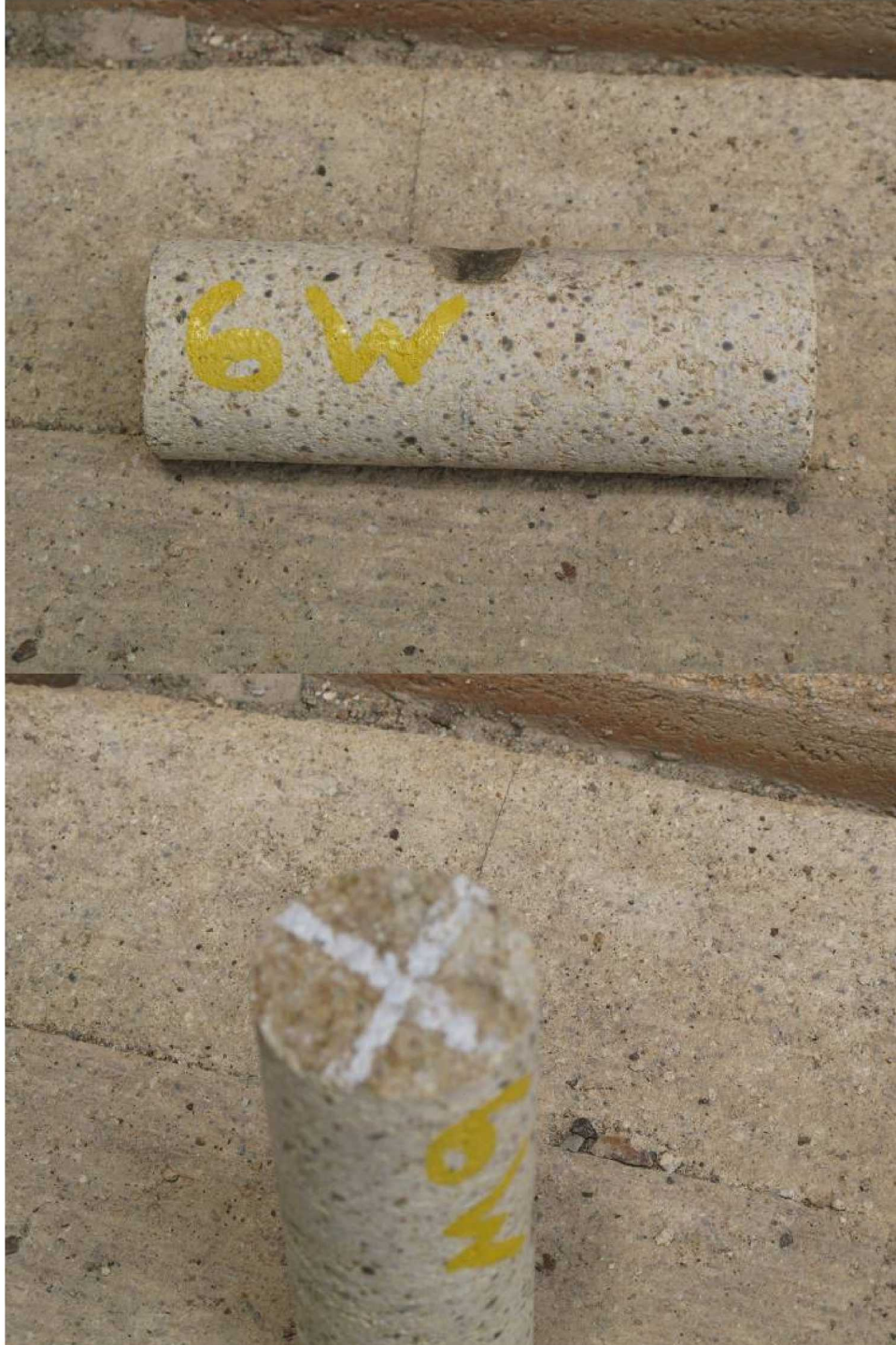
Figure 30. Core 6W – side image of core and outer surface of core removed during core drilling
