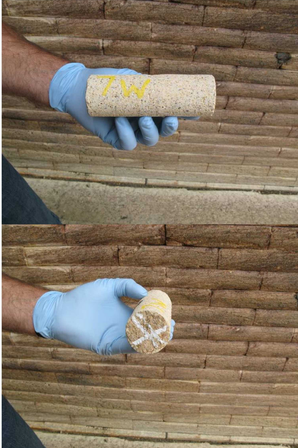
Figure 32. Core 7W – side image of core and outer surface of core removed during core drilling
