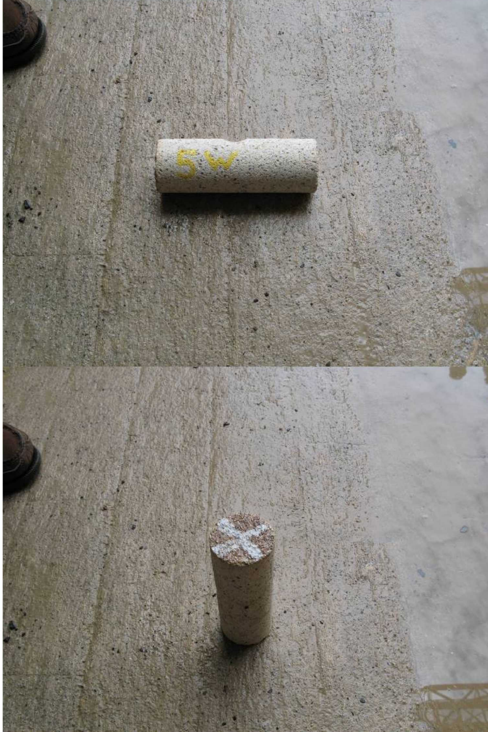
Figure 28. Core 5W – side image of core and bottom outer surface of core removed during core drilling
