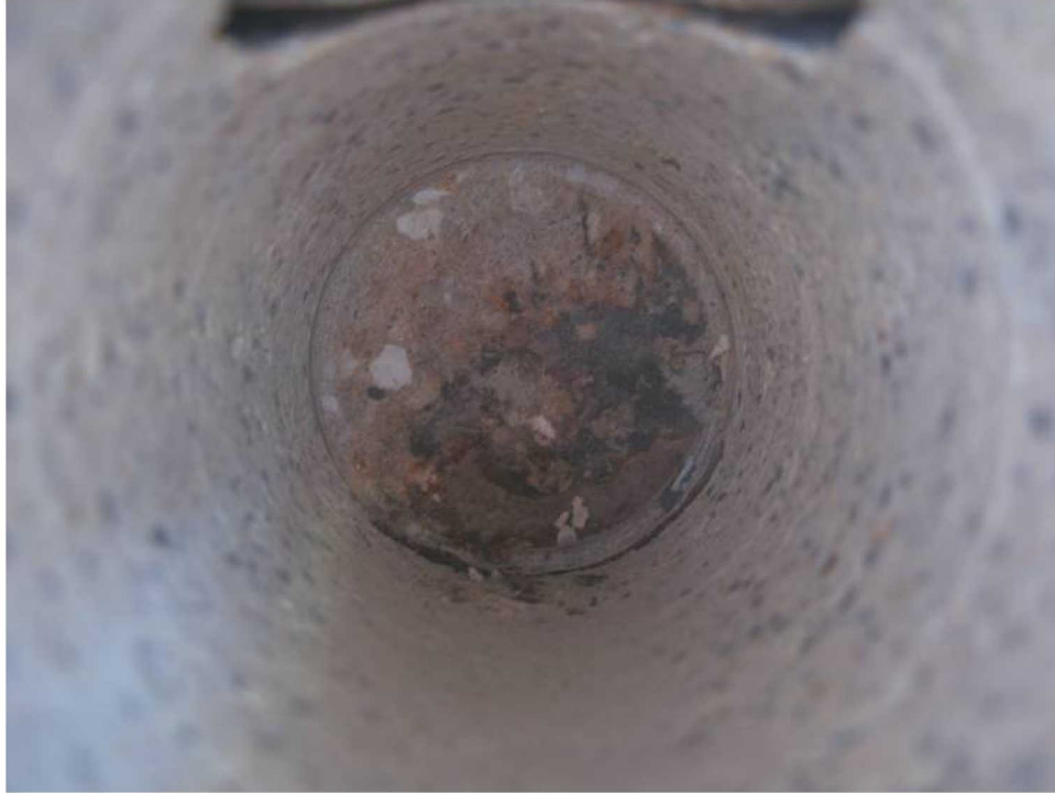
Figure 35. Core 8W – inside the brick after the core was removed
