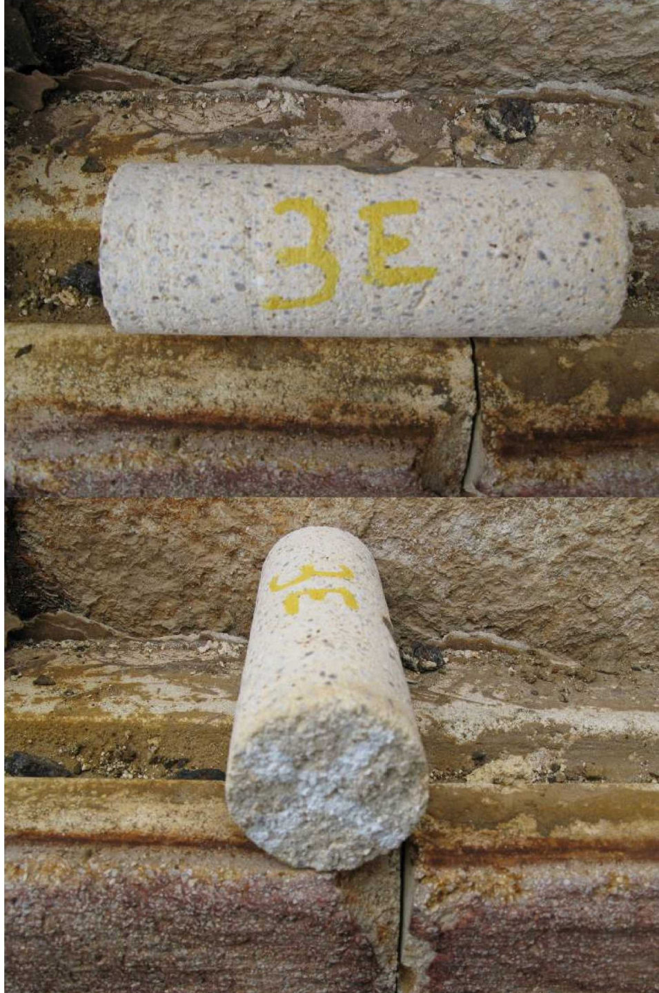
Figure 12. Core 3E – side image of core and outer surface of core removed during core drilling
