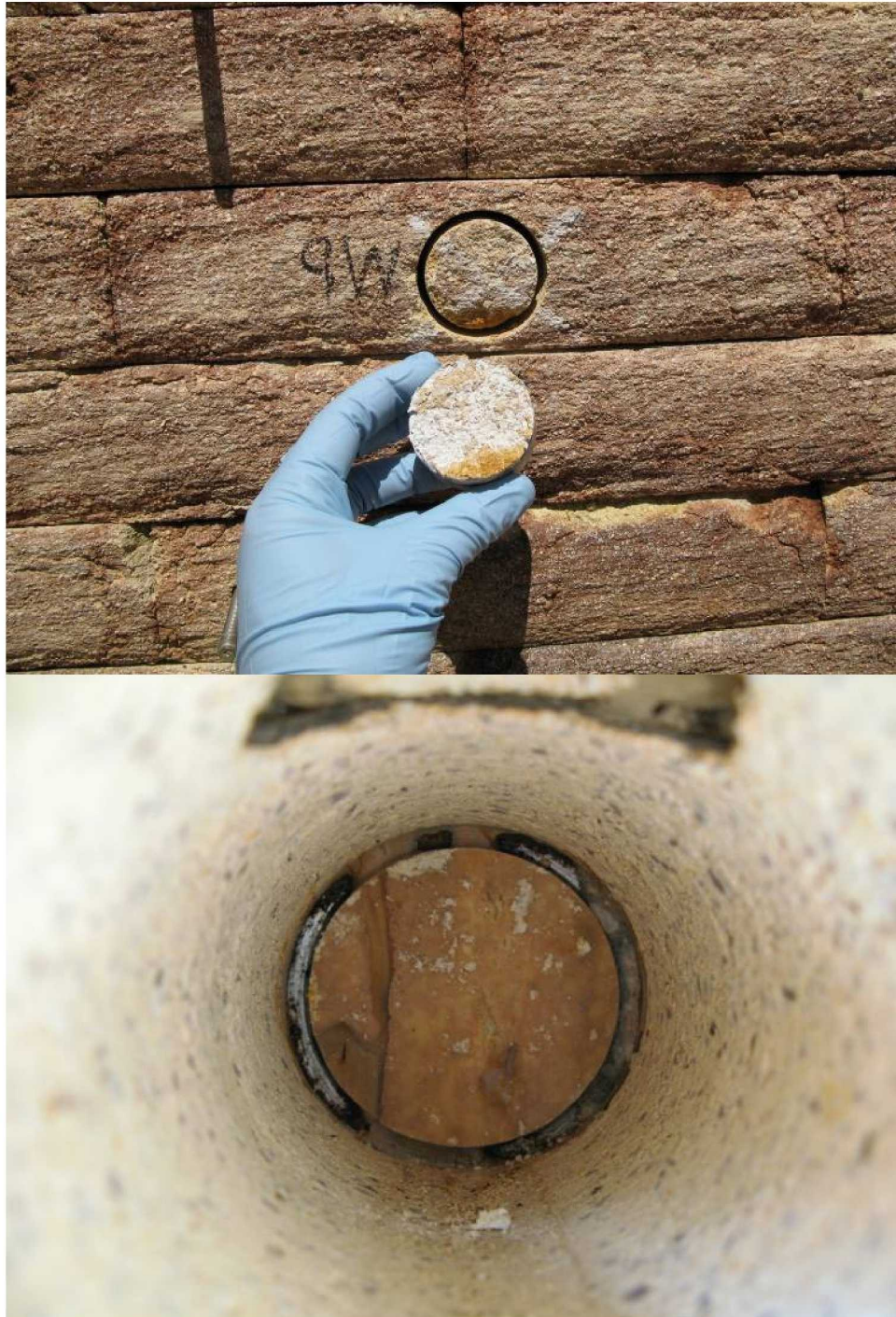
Figure 37. Core 9W – successful test: failed at 54 psi (pull stub and core face and inside the brick after the core was removed)
