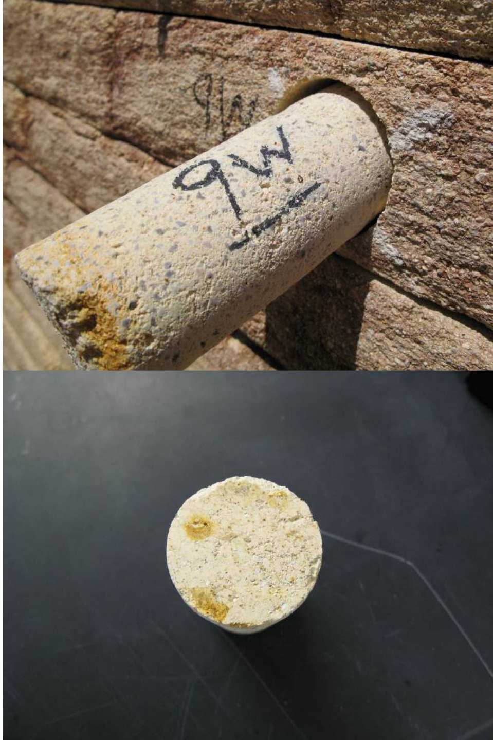
Figure 36. Core 9W – side image of core and back end of core, closest to the concrete wall
