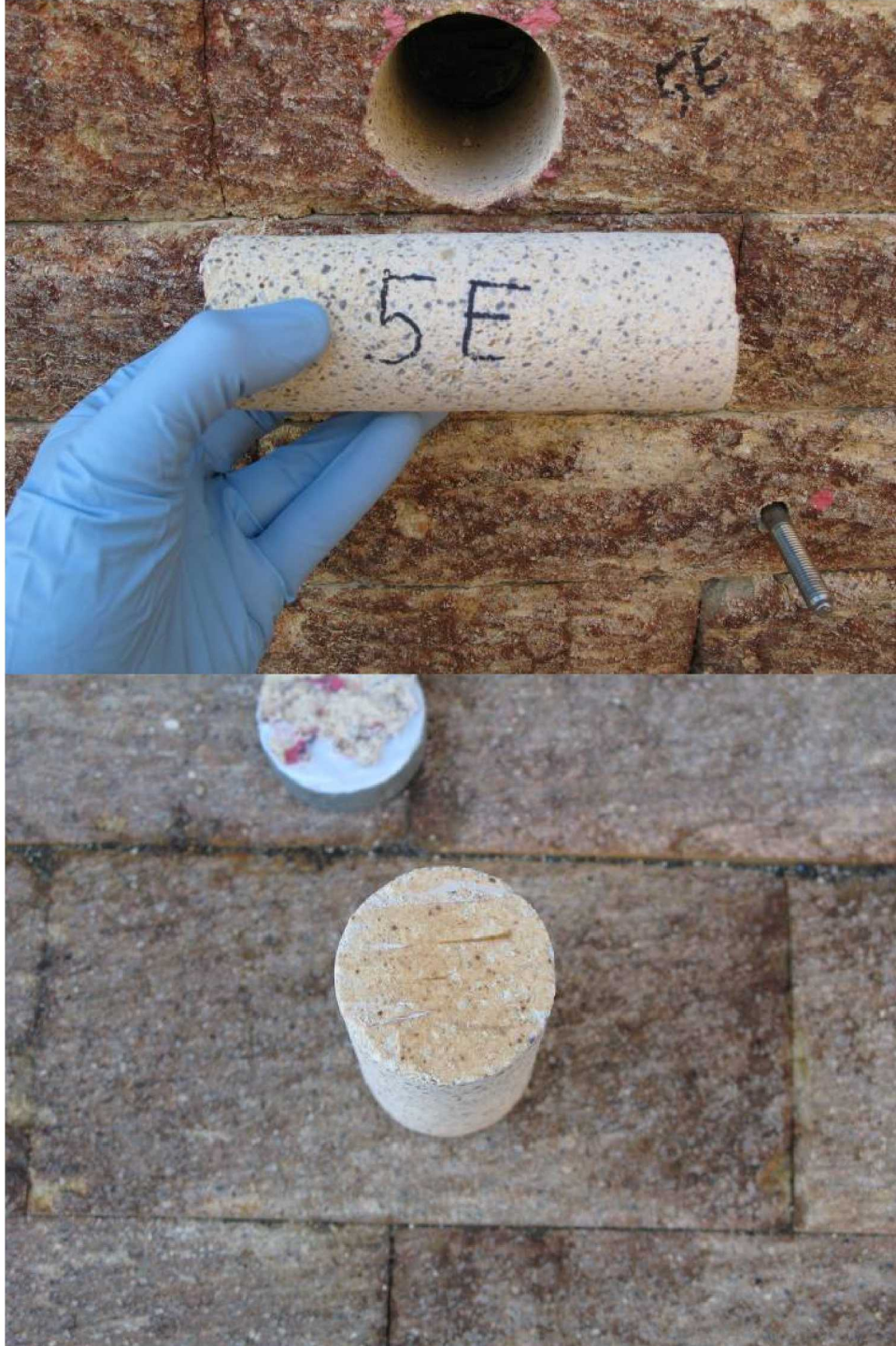
Figure 16. Core 5E – side image of core and back end of core, closest to the concrete wall
