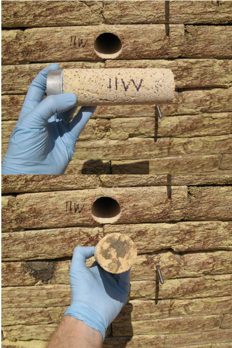
Figure 40. Core 11W – side image of core and back end of core, closest to the concrete wall
