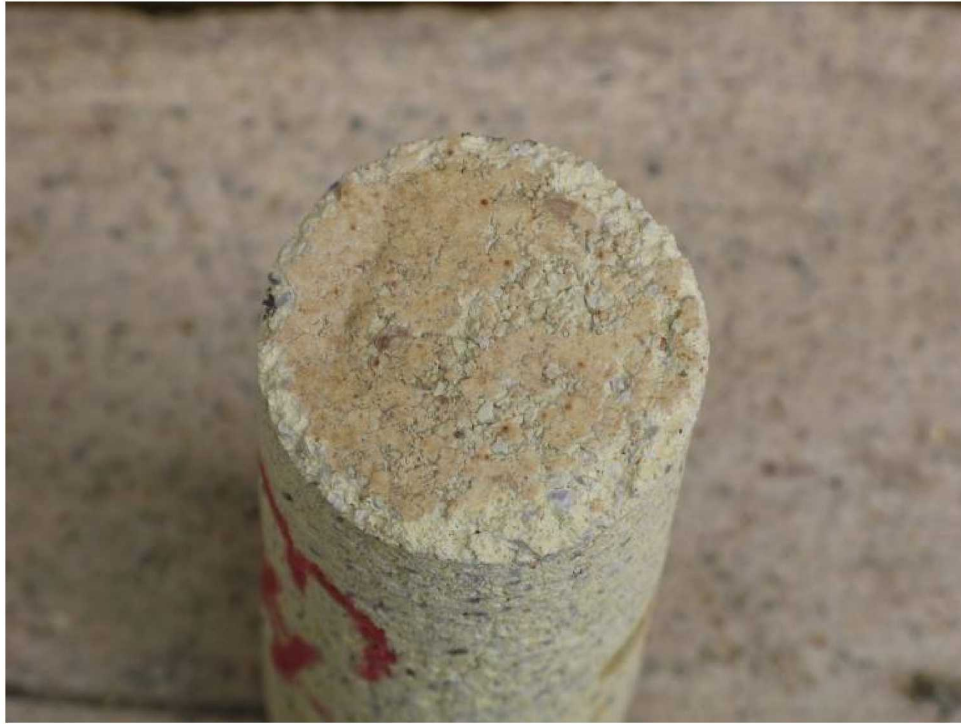
Figure 25. Core 3 – inner surface of core removed during core drilling
