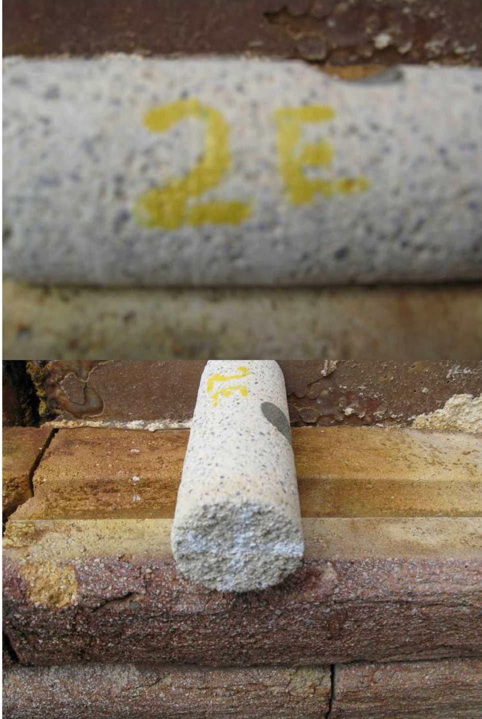
Figure 10. Core 2E – side image of core and outer surface of core removed during core drilling
