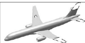
Considered GTM Damages
