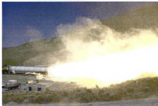
Figure 2. Four-segment RSRB static test firing, April 2006.
