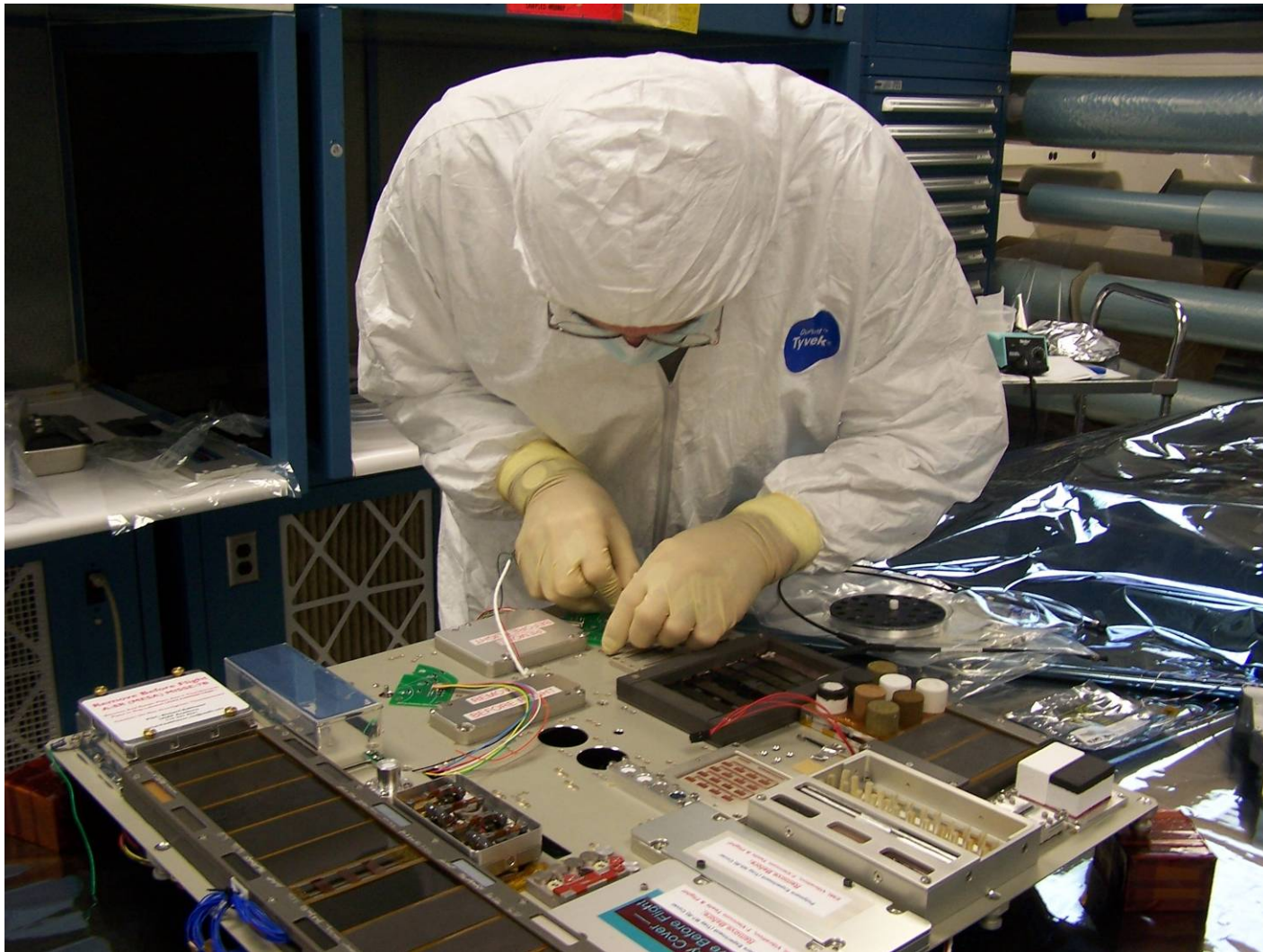
Andy Robb installing the Hall sensor boards
