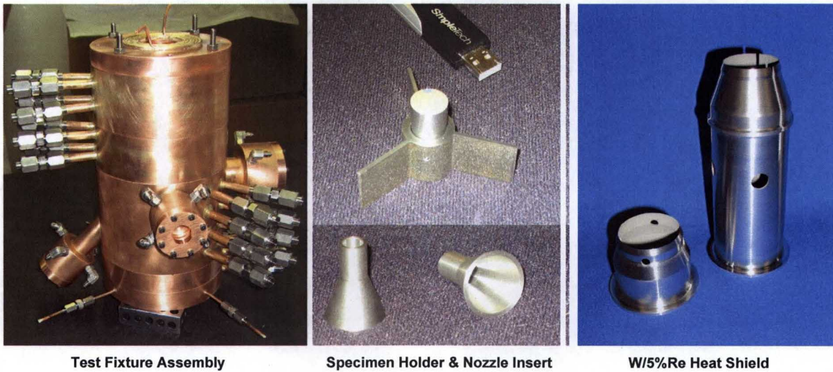
Figure 7. Photographs of fabricated test fixture hardware and refractory metal alloy components.
