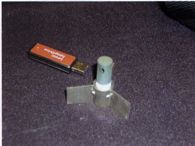
Figure 20. CERMET specimen with black body cavity.
