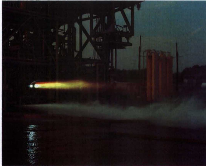
Figure 11. Subscale 40-element injector test at MSFC.
