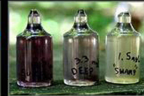
Prepared sampling vials can be used to measure dissolved oxygen concentrations
