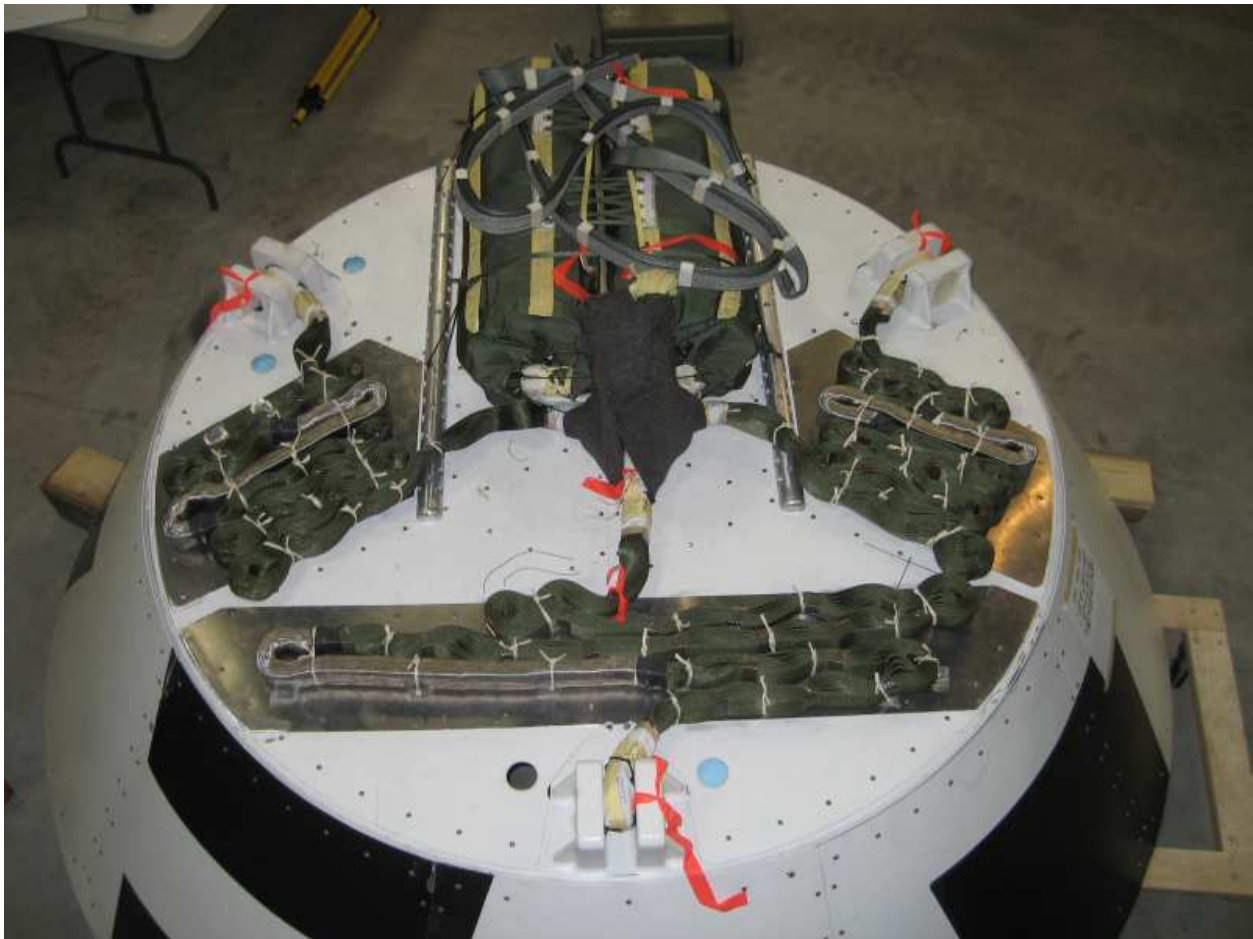
Figure 6. FBC Drogue Installation
