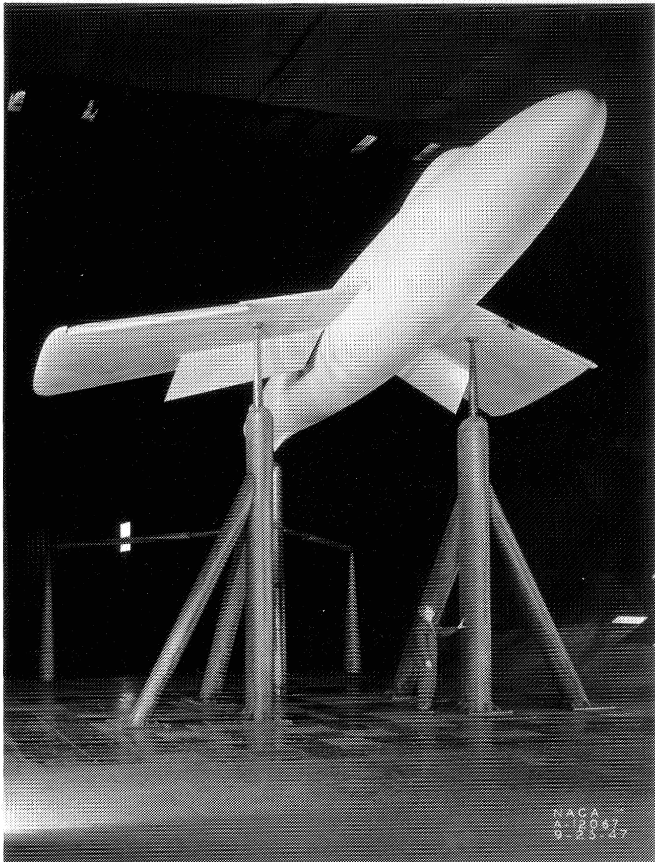
Figure 6.- The wing-fuselage installation in the Ames 40- by 80-foot wind tunnel; partial-span drooped slats and split flaps extended.
