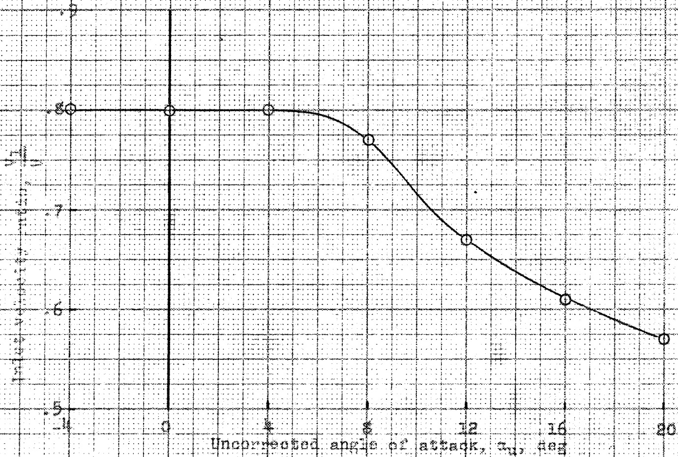
Figure 5. Inlet flow characteristics with engine removed. V = 126 mph
