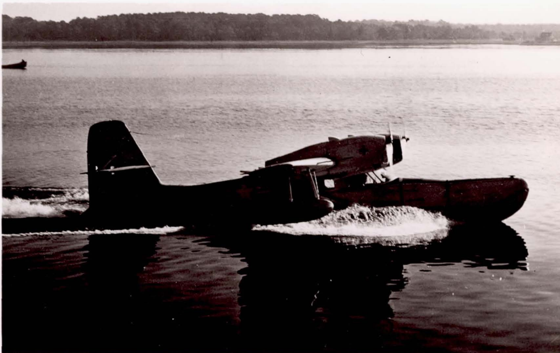
(a) Wing-high side; center of gravity, 25 percent M.A.C.
