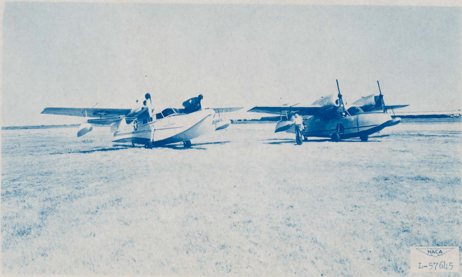
Figure 2.- Three-quarter front view of J4F-2 with 0.425-scale XP5M-1 hull bottom and standard J4F-2.
