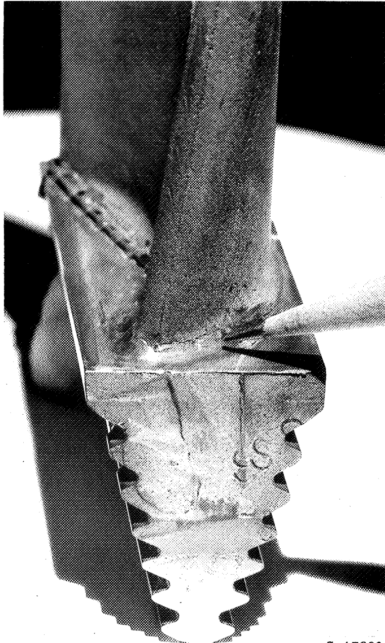
Figure 8. - Crack at junction of porous shell and base platform of blade 38.
