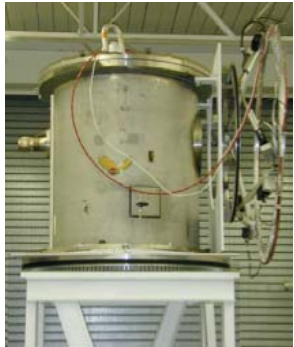
Figure 4. Vacuum Chamber with mounting plate and gimbal platform.
