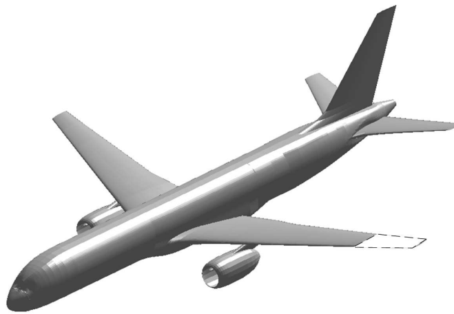
Fig. 5 - Damaged Generic Transport Model
