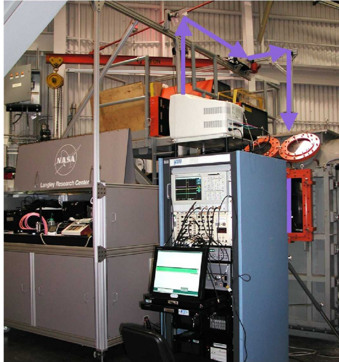
Figure 3. Photograph of the laser cart and electronics rack installed in the 15-inch Mach 6 wind tunnel facility. The test section is visible behind the electronics rack. Arrows indicate the path of the laser beam.
