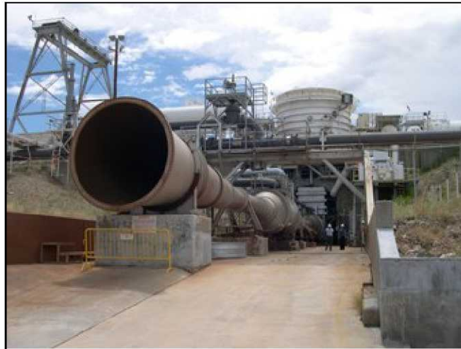
Figure 2: WSTF TS-401 with LASS ejector exhaust shown.
