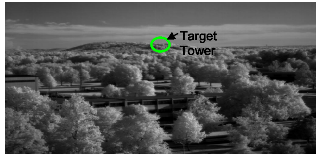
Figure 12: Image taken from NGAVGS of 5 km target area during daytime. Target tower is barely visible.
