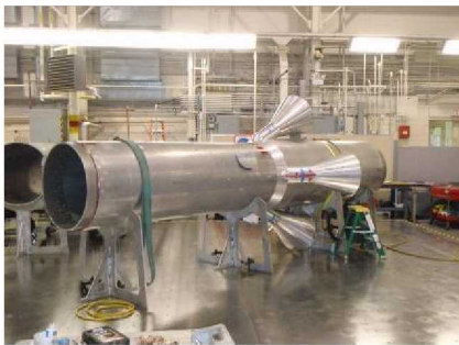
Figure 11. The launch abort system (LAS) simulator during assembly at Langley Research Center.
