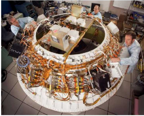
Figure 19. The Ares I-X avionics undergoing testing in the Systems Integration Laboratory.
