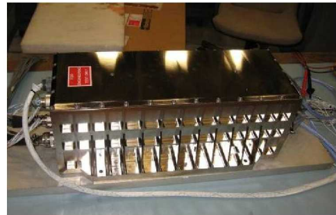
Figure 18. The ascent thrust vector controller (ATVC) communicates between Atlas V and Space Shuttle hardware to send steering commands to the first stage nozzle.
