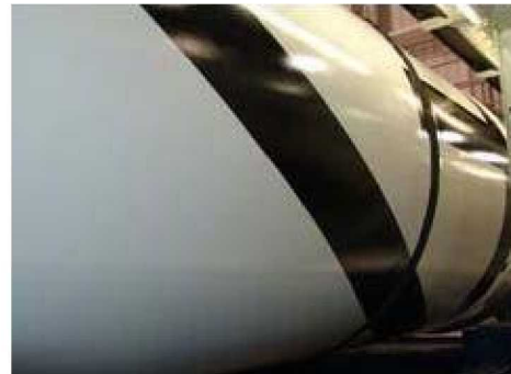
Figure 6. Close-up image of motor segment with completed Z-stripe.
