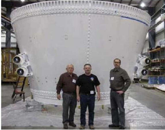
Figure 7. The frustum connects the first stage to the wider upper stage simulator.
