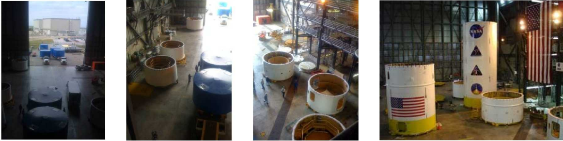
Figure 10. The upper stage simulator segments in the process of delivery (far left), unpacking (middle), and stacking (far right).
