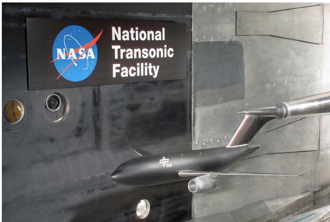
Figure 4. Photograph of the DLR-F6 model mounted in the test section of the National Transonic Facility.
