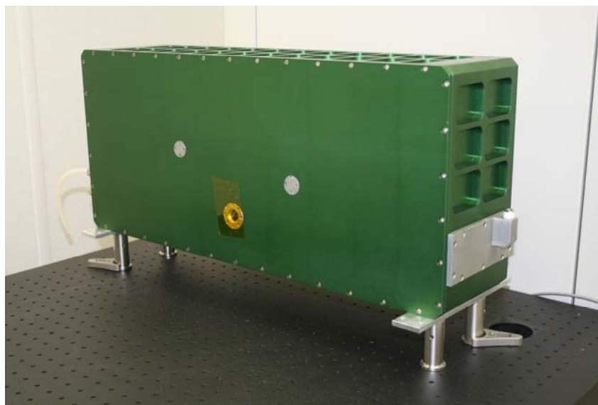
Figure 2. The DAWN pulsed, 2-micron, coherent Doppler wind lidar transceiver
