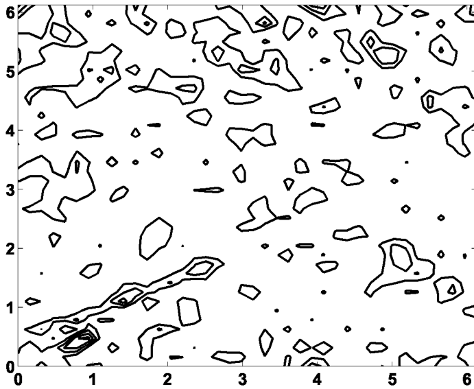
Figure 3: Contour plot of analysis field minus true field ( \mathbf{c}^a - \mathbf{c}^t ) at the end of 1000 timesteps. The contour levels are 0.3. The largest errors are around 0.7, and occur near the source term ( x = 0.47, y = 0.47 ).
