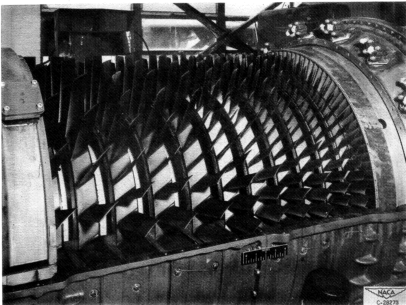
Figure 3. - View of compressor with top half of casing removed.
