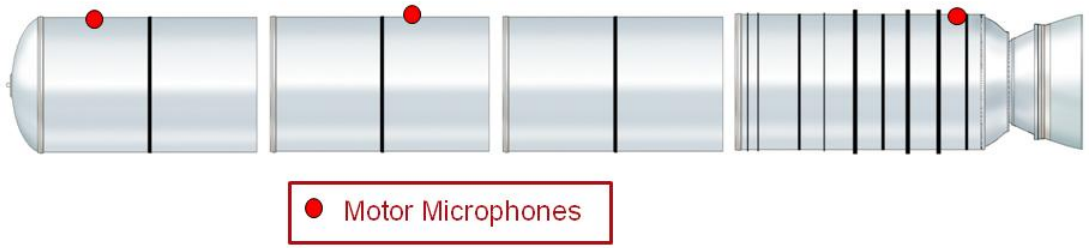
Figure 1. RSRM on-motor microphone layout
