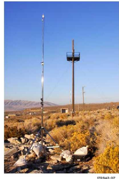
Figure 5. Acoustic microphone tripod setup.
