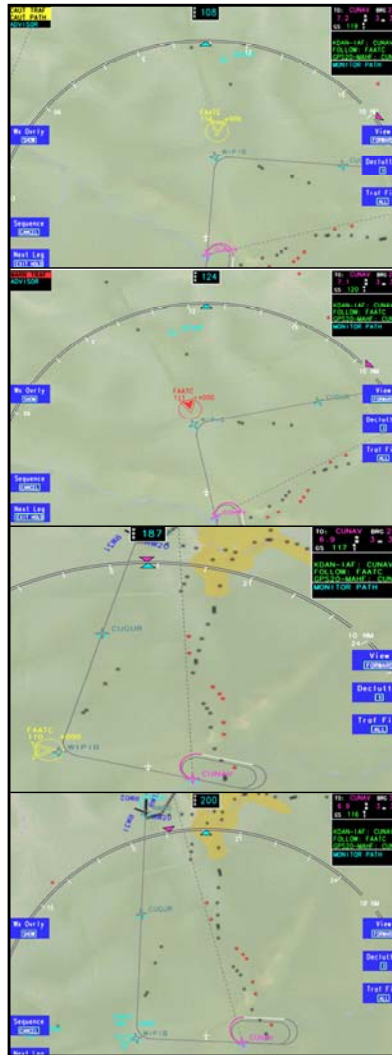
Figure 5: Multi-level Alerting During Approach Sequence
