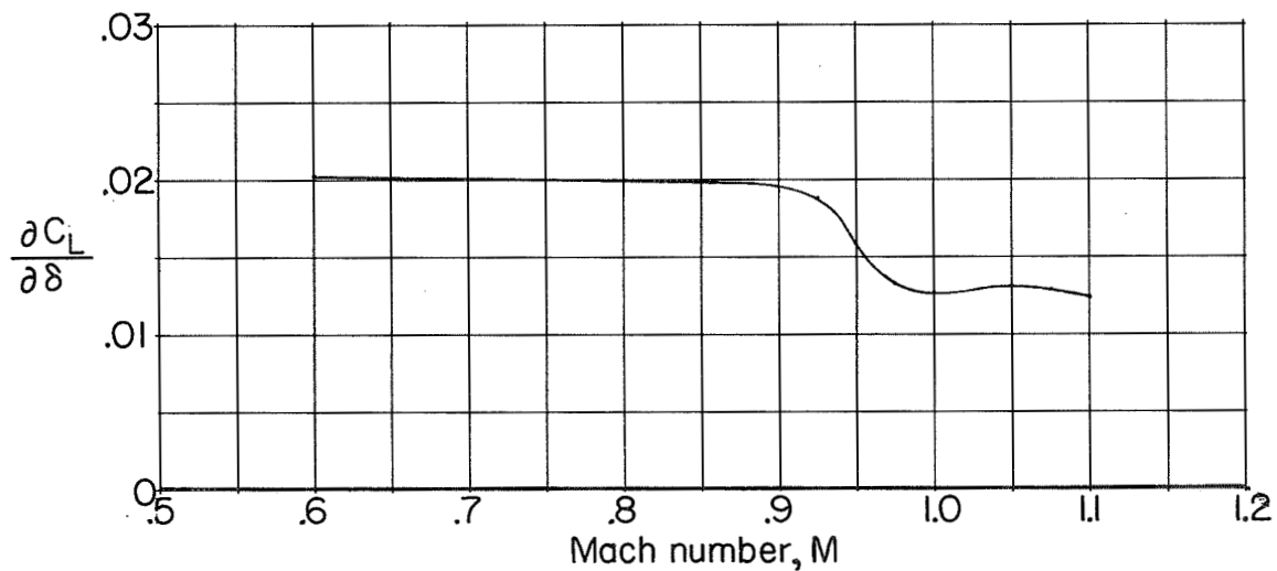
Figure 9.- Variation with Mach number of the lift-curve slope and the elevator lift effectiveness parameter.
