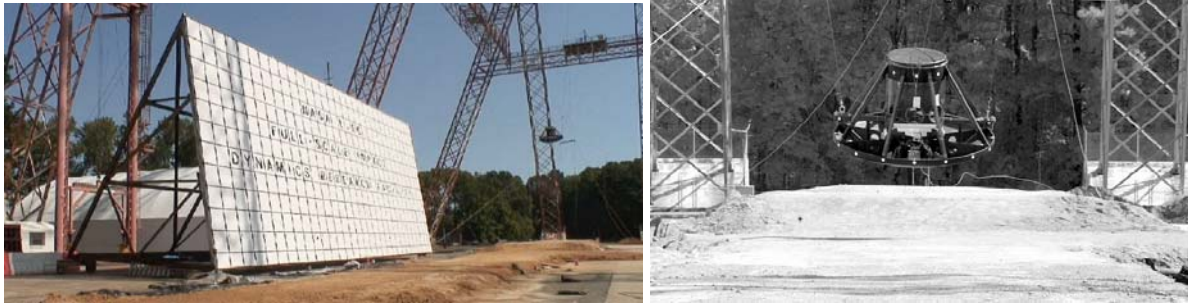
Figure 11. Boilerplate swing test at the NASA Langley LandIR facility.
