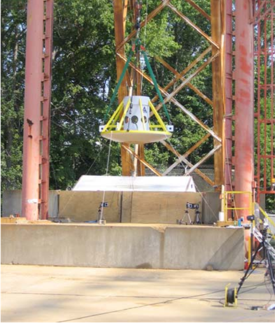
Figure 19. First vertical drop test of boilerplate into flat soil impact surface using the vertical drop tower at LandIR.
