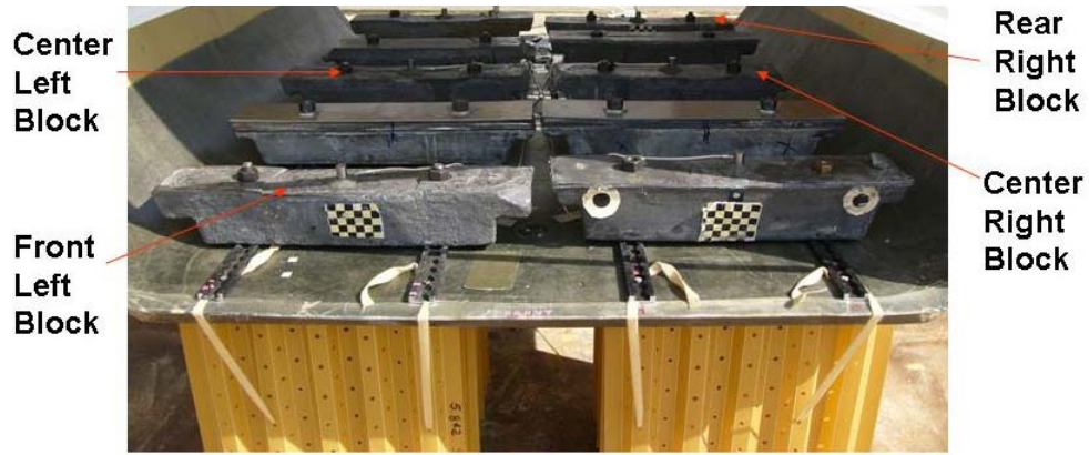
(a) Test article with accelerometer location labels taken for analysis correlation.
