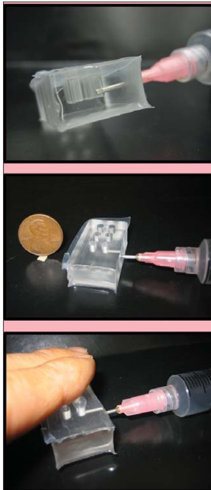
A Syringe Is Used to pump air into one of the holes in the block, causing the portion of the sheet covering that hole to protrude to provide a tactile sensation.
