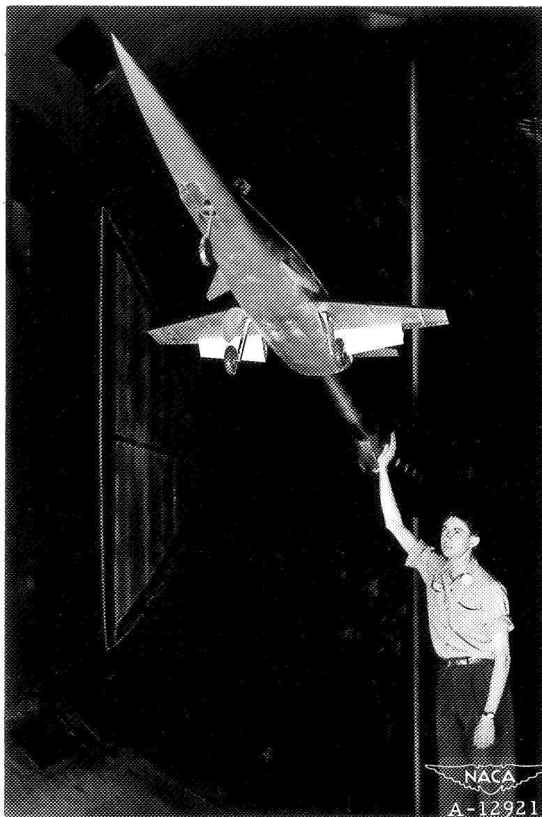
Figure 2.— A three-quarter front view of the MX-656 model with the landing gear extended, the flaps deflected, and the nose fins in the normal position.
