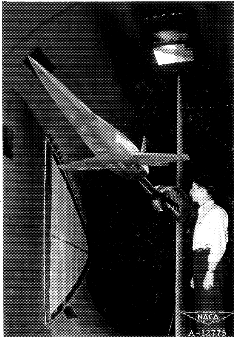
Figure 2. - The MX-656 model mounted in the Ames 16-foot high-speed wind tunnel for pressure-distribution tests in pitch.
