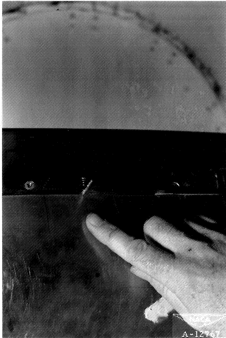
Figure 4.- The fuselage boundary-layer rake mounted on the MX-656 model.
