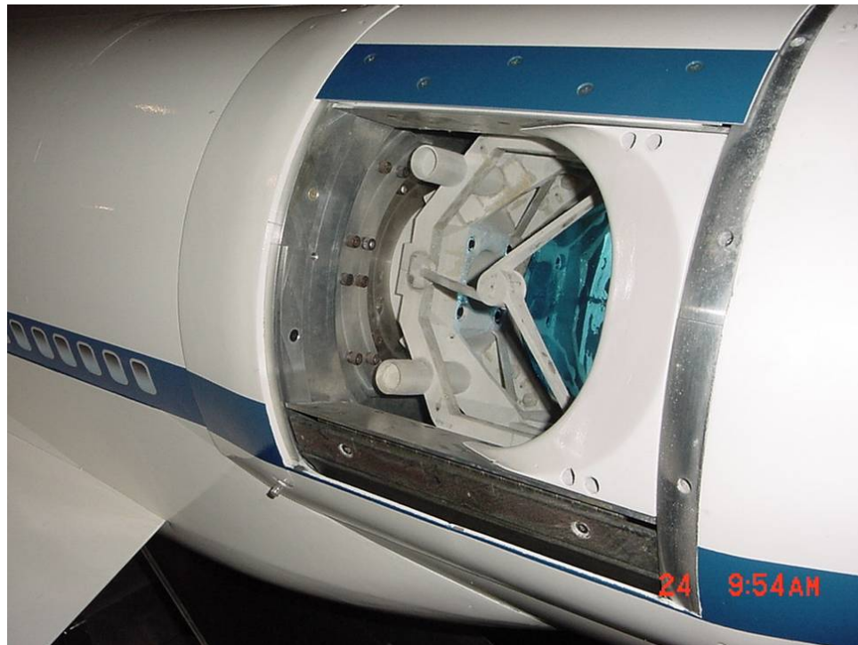
Figure 6.2.1-1. Seven Percent Wind Tunnel Model Telescope Assembly Cavity
