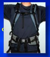
Evaluation of a new treadmill harness design for comfort during exercise, and measurement of the loads in the harness straps for direct comparison with the current U.S. TVIS Harness. The research protocol is aimed at improving comfort, plus increasing consistent loading for crewmembers exercising on the ISS treadmill.
