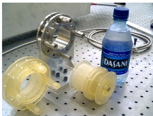
Figure 9. Prototypes of single-stage air compressor assembly (Impeller, IGV and diffuser) and housing
