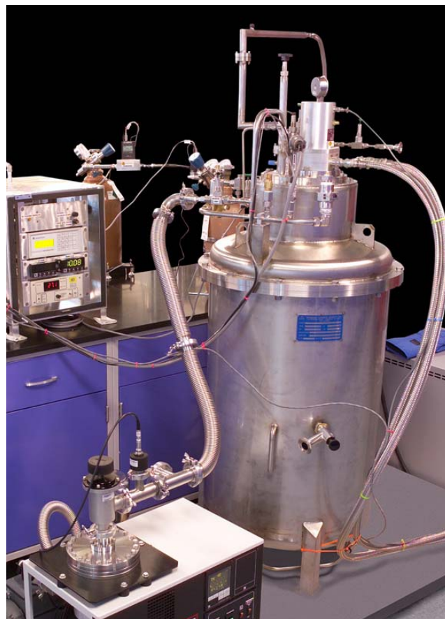
Figure 1. A 150 liter liquid hydrogen densification and zero-boil-off storage system at FSEC.
