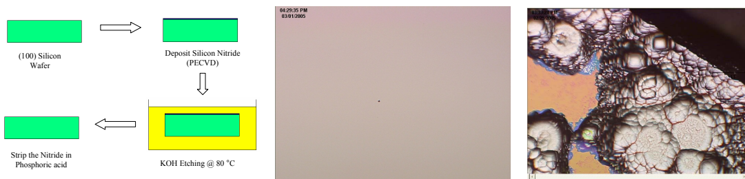
Figure 1(a). Process for testing the porosity of silicon nitride thin film, (b) Smooth surface of silicon nitride, (c) Etched pitted surface.
