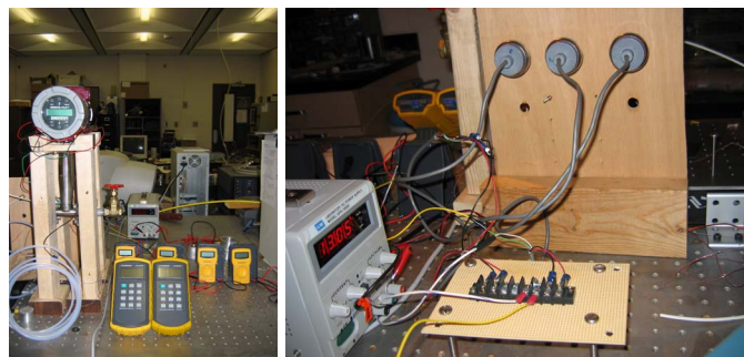
Figure 58. Mass flow meter, thermocouple units, pressure transducers and multimeters
