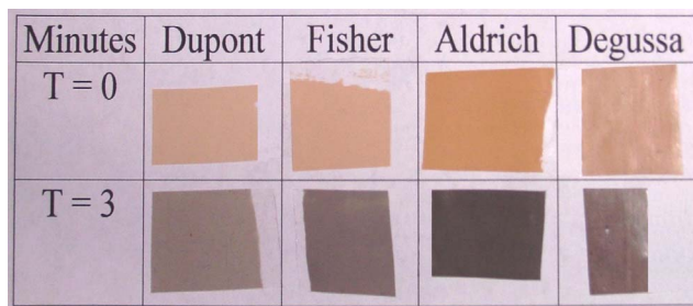
Figure 10. Comparison of pigment formulations exposed to hydrogen.
