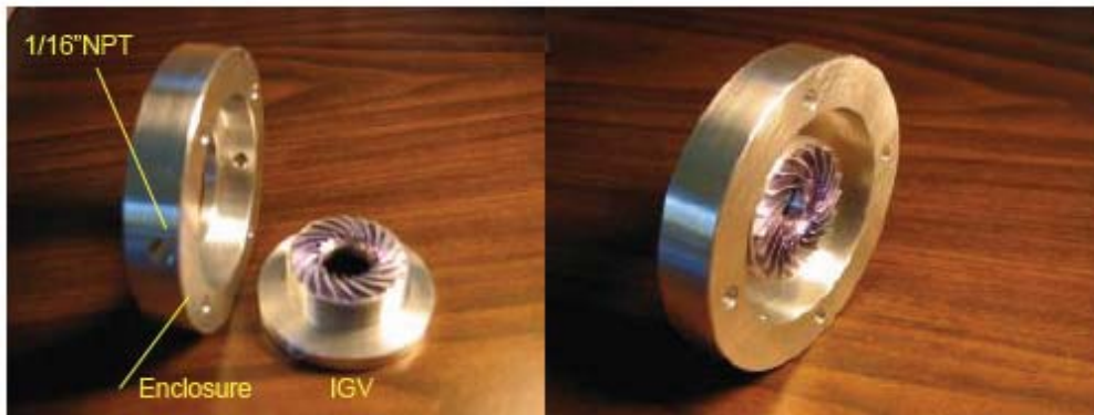
Figure 53. Gas passage and IGV
