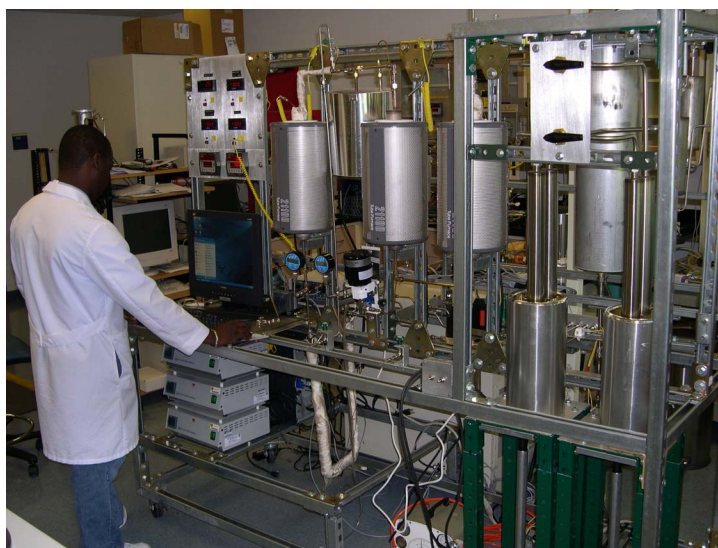
Figure 11. Hydrogen production unit with the capacity of 1 SCFM.
