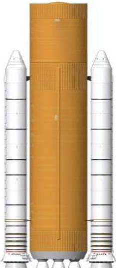
Core Stage LOx/LH 2 6 RS-68B Engines Al-Li Tanks Composite Structures
