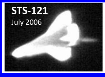
STS-121 July 2006 Turbulent flow from gap filler ~ Mach 13 Horvath et. al. AIAA-2007-4267
