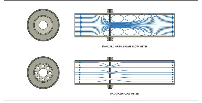
The Flow in the Balanced Flow Meter is straighter and less turbulent. One consequence is the net pressure loss downstream for the balanced flow meter is less than half that of the standard orifice-plate flow meter.
